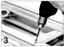
Using the bit provided, drill all 4 holes. Use a center punch to ensure accuracy of holes.
