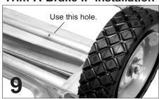
To install wheel kit on Trim-A-Brake II<sup>®</sup> models, use inner cotter pin hole. Trim excess axle shaft using a hacksaw.
