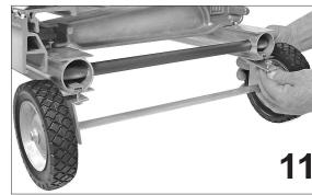
Slide the screw heads into the slots on each side. With the ends of the brackets flush to the ends of the base rail, tighten all hex nuts firmly in place with a 7/16" wrench.
