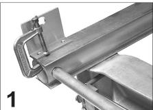
Turn brake over and decide which end to mount the wheel kit. As shown above, clamp the bracket even with the rail.
