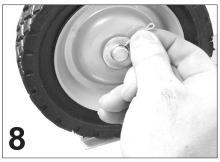
Insert Cotter pin through hole in shaft end and spread apart to prevent pin from dislodging from hole.
