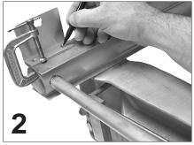
Mark each hole with a pencil and remove clamp. Repeat step 1 and 2 with remaining bracket and again remove clamp.
