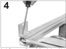
Install screws through bracket and into base rail using a Phillips screwdriver. Repeat step with other bracket to rail.
