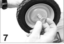
Slide washer onto axle shaft until cotter pin hole is clearly visible (Trim-A-Brake, or I-Beam see Step 9 first).
